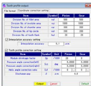
Fig. 4.48 Coordinate correction setup
